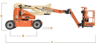
A. Platform Width 30-in / 76-cm B. Platform Length 48-in / 1.22-m C. Machine Width 4-ft 11-in / 1.5-m 4-in / 10-cm E. Machine Height 6-ft 5.75-in / 1.97-m F. Machine Length 22-ft / 6.71-m 6-ft 7-in / 2.01-m H. Ground Clearance 5-in / 13-cm
