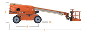
Platform Width 36-in / 0.91-m B. Platform Length 96-in / 2.44-m C. Machine Width 8-ft 2-in / 2.48-m D. Tailswing 4-ft / 1.22-m Machine Height E. 8-ft 2.4-in / 2.50-m F. Machine Length 28-ft 7-in / 8.71-m G. Wheelbase 8-ft 2.7-in / 2.5-m H. **Ground Clearance** 11.3-in / 29-cm
