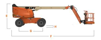
Platform Width 36-in / 0.91-m Platform Length 96-in / 2.44-m Machine Width 7-ft 6.8-in / 2.31-m C. Tailswing 3-ft .5-in / 93-cm D. Machine Height 8-ft 1-in / 2.47-m E. E. Machine Length 29-ft 8.2-in / 9.10-m Wheelbase 7-ft 9.5-in / 2.37-m G. **Ground Clearance** 12-in / 30-cm H.
