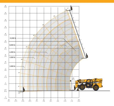
These load charts are for the rated capacity of the machine with 66" wide standard carriage and 48" pallet forks. Use only JCB approved attachments and check the relevant load chart for the machine model.
